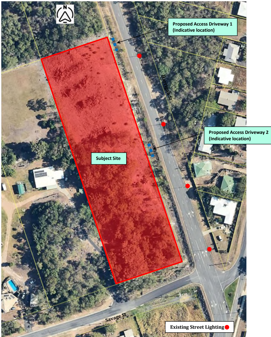
Figure 18 – Existing Street Lighting (Source: QLD Globe)
