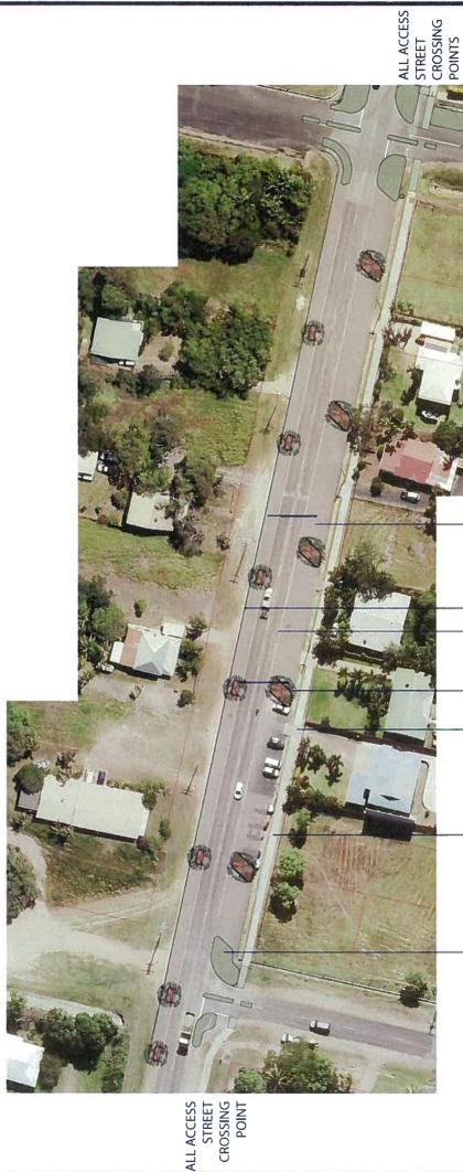
REDESIGNED REALIGNMENTS TO INTERSECTION TIE BACK TO EXISTING NEW KERB & CHANNEL CONTINUOUS TO WESTERN SIDE - SEALED PARKING
