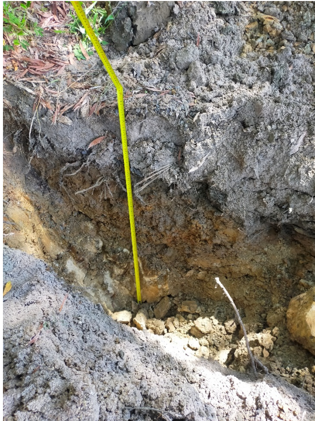
PHOTOGRAPH 2: View of soil profile of Test Pit 1
