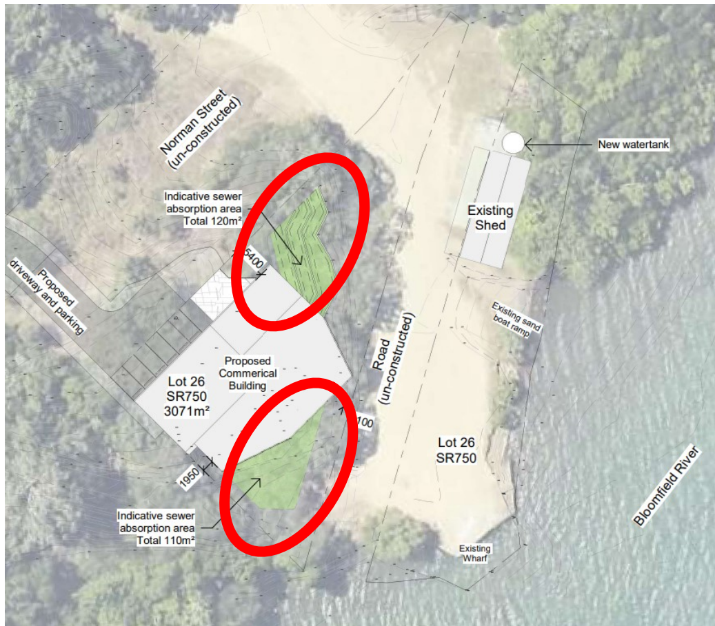
Image # 3 – Two Portions of Lot 26 on SR750 with Effluent Disposal Area Shown Circled
